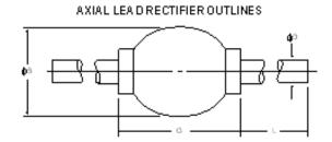
**Termination Finish:** Axial leads and Endcaps are copper with Tin/Lead finish.
