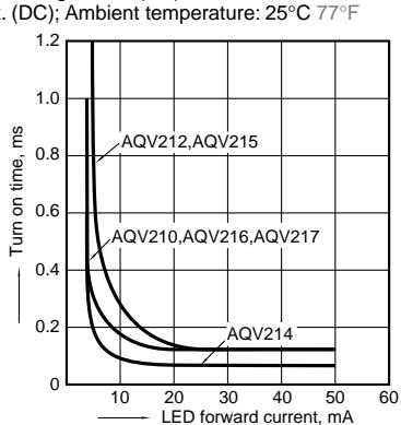
**10-(2). LED forward current vs. turn on time characteristics**
