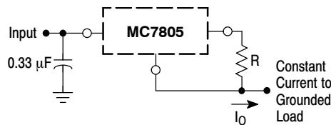
The MC7800 regulators can also be used as a current source when connected as above. In order to minimize dissipation the MC7805C is chosen in this application. Resistor R determines the current as follows:
