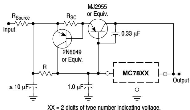
The circuit of Figure 10 can be modified to provide supply protection against short circuits by adding a short circuit sense resistor,  $R_{SC}$ , and an additional PNP transistor. The current sensing PNP must be able to handle the short circuit current of the three-terminal regulator. Therefore, a four-ampere plastic power transistor is specified.
