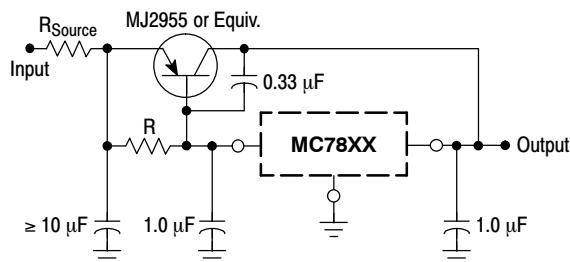
The MC7800 series can be current boosted with a PNP transistor. The MJ2955 provides current to 5.0 A. Resistor R in conjunction with the  $V_{BE}$  of the PNP determines when the pass transistor begins conducting; this circuit is not short circuit proof. Input/output differential voltage minimum is increased by  $V_{BE}$  of the pass transistor.
