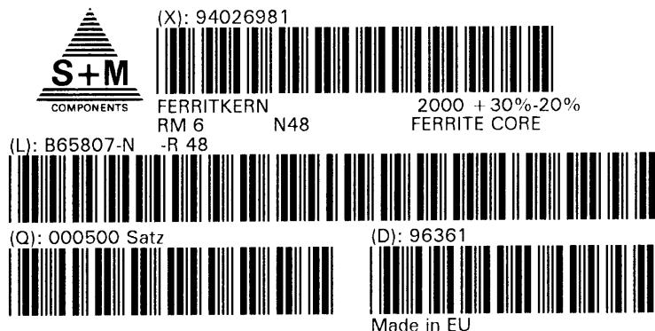
The date code (D) indicates the quality assurance release date, which enables the respective production batch to be traced back to the respective production stage.
